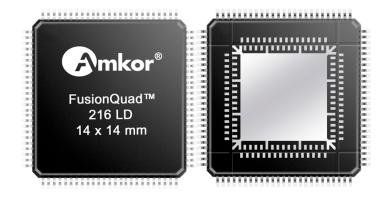
FusionQuad<sup>TM</sup> offers a unique blend of excellent <u>electrical</u> and <u>thermal</u> performance in a miniaturized cost-effective leadframe plastic package. The unique footprint of FusionQuad<sup>TM</sup> allows for the use of low cost printed circuit boards in the end application due to the space available for coarse routing vias between the bottom lands and the outer peripheral leads.
